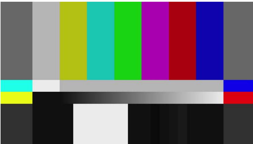
Figure 2: SMPTE RP-219-2002 test pattern available from the module
