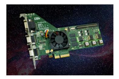
For optimal image acquisition, Active Silicon's FireBird Camera Link 80-bit frame grabber was chosen along with a 10m passive Camera Link cable also supplied by Active Silicon which was critical to the project.
