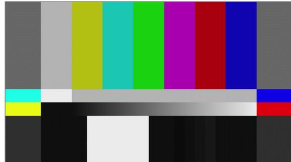
Figure 4. Static Test Pattern (DIP switch 1 ON)
