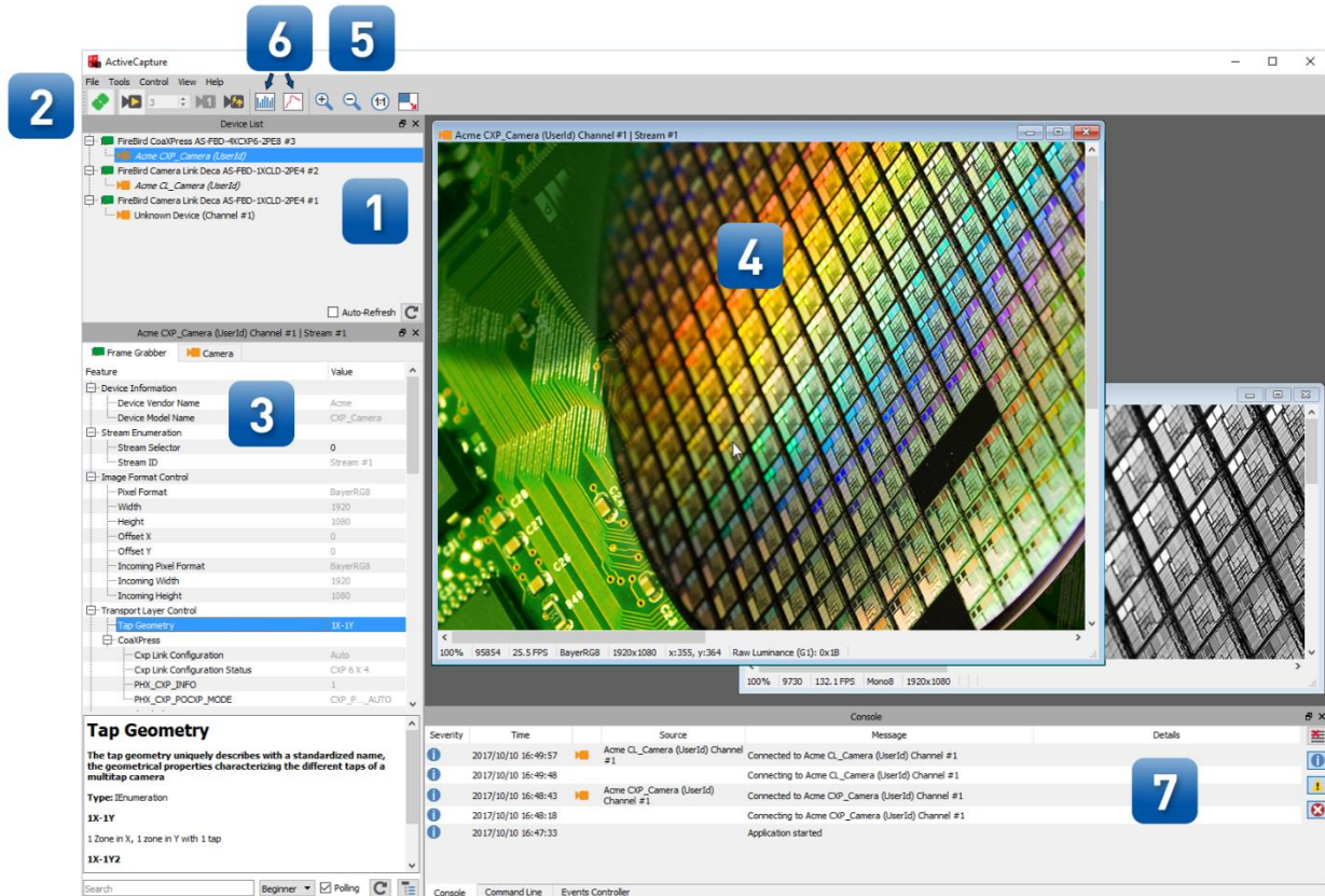
Fig. 1. The graphic user interface – the example shows three frame grabbers, each connected to one camera.
