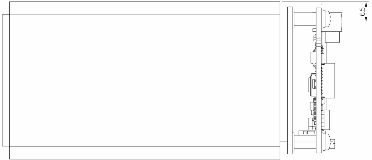
Figure 5: Board attached to EV7500 camera (top view).
