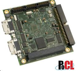
**Phoenix-D48CL** supports the Power over Camera Link (PoCL) functionality with *SafePower* and is able to provide power to PoCL enabled cameras via the Camera Link data cable thereby removing the need for a separate power supply. Conventional non-PoCL cameras are still supported.
