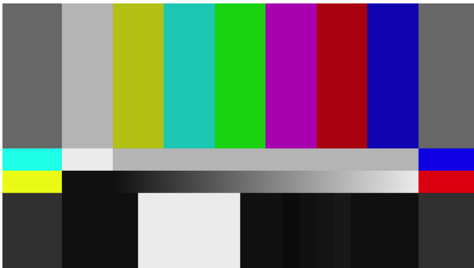
Figure 2: SMPTE RP-219-2002 test pattern available from the interface board.
