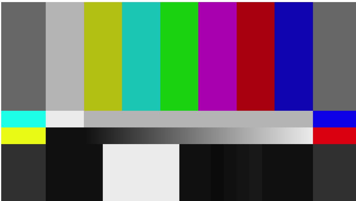
Figure 3. SMPTE RP-219-2002 test pattern available from the interface board.
