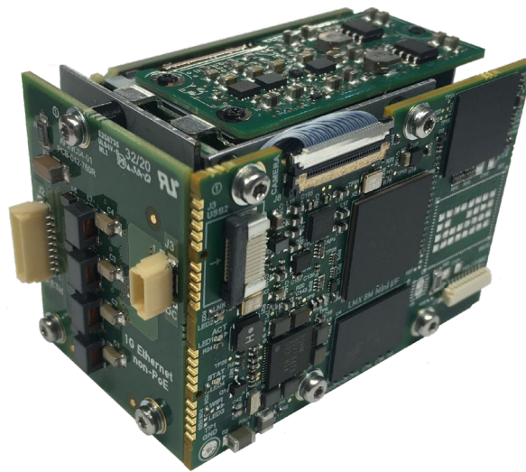
Figure 1. Harrier Ethernet Connection Board (IFETH) mounted on the back of a Tamron MP1010M camera with the Harrier IP Camera Interface Board (SoC board) on the side.
