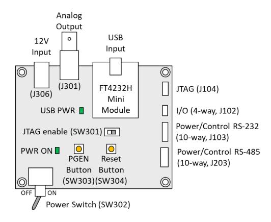
Figure 1. Harrier Evaluation Board diagram
