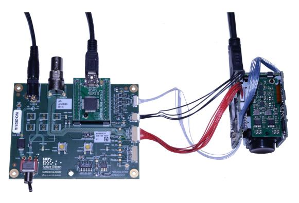
Figure 2. Harrier Evaluation Board in use with a Harrier Camera Interface Board and Tamron camera
