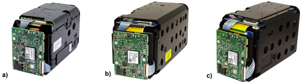
Figure 2. Camera assemblies with rear mounted Harrier HDMI Camera Interface Board a) Harrier 30x AF-Zoom HDMI Camera (Sony FCB-EV7520), b) Harrier 36x AF-Zoom HDMI Camera (global shutter), c) Harrier 40x AF-Zoom HDMI Camera.
