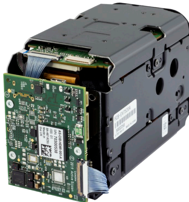
Figure 2. Harrier HDMI Camera Interface Board mounted on a Sony FCB-EV7520A camera.
