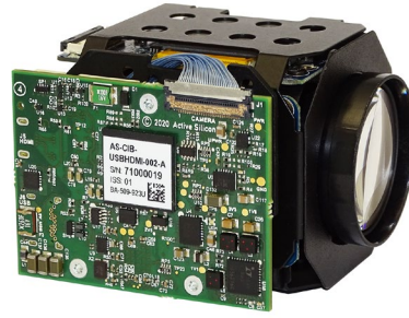
Figure 1. Harrier 10x AF-Zoom HDMI Camera – a camera assembly with side mounted Harrier HDMI Camera Interface Board.
