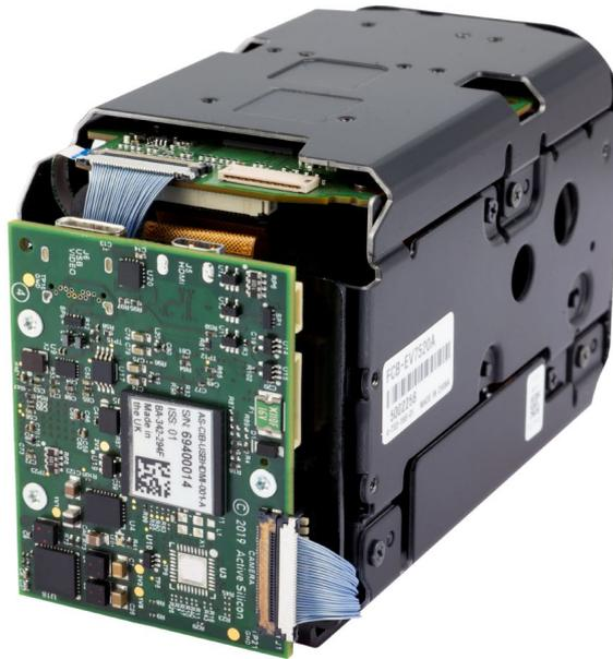
**Figure 1. Harrier USB/HDMI Camera Interface Board mounted on a Sony FCB-EV7520 camera.**
