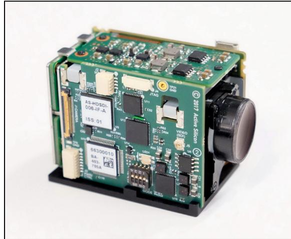
Harrier Interface Board fitted to camera
