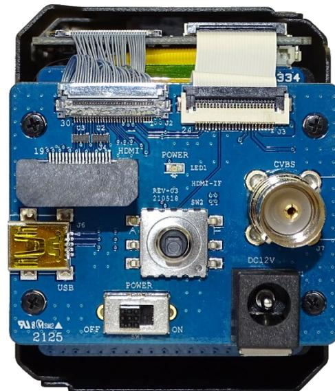
**Figure 3. Harrier 18x HDMI 4K Camera Evaluation Board mounted on the camera.**
