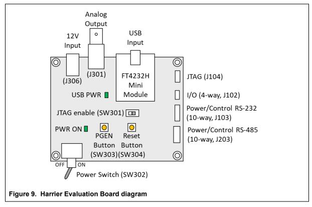
The Harrier Evaluation Board connects to the camera interface board using the supplied cable kit.
