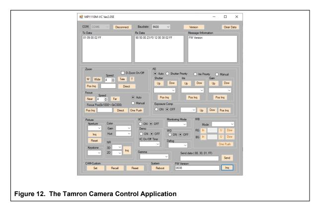
When the Harrier Evaluation Board is plugged in using the mini USB cable, the Windows operating system will see three virtual COM ports; these ports are automatically assigned (incrementing) numbers by Windows. To successfully use the Tamron application, it is necessary to identify the COM port numbers which Windows has assigned to the board and use the correct one.
