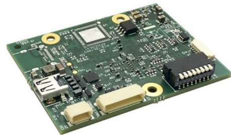
Figure 2. Reverse side of Harrier HDMI Camera Interface Board.
