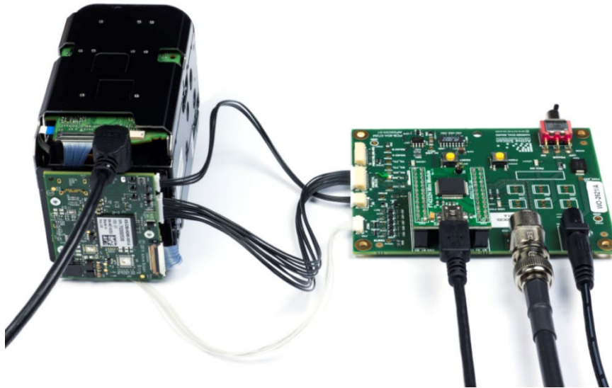
Figure 8. Harrier Evaluation Board connected to the Harrier HDMI camera interface board and Sony FCB-EV7520A camera
