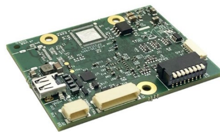
Figure 3. Reverse side of Harrier HDMI Camera Interface Board.
