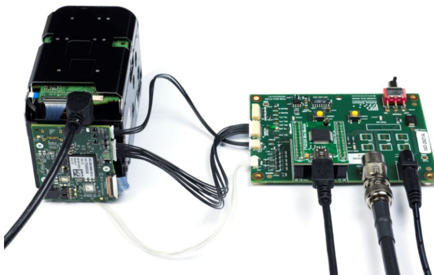
Figure 9. Harrier Evaluation Board connected to Harrier HDMI Interface Board module and A) a Tamron MP1010M camera, B) a Sony FCB-EV7520A camera.
