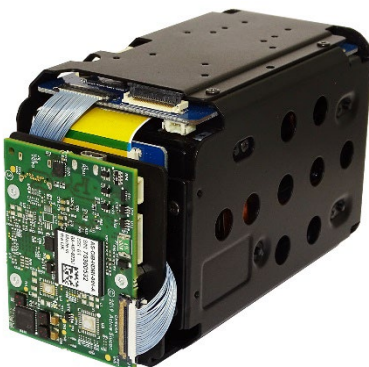
Figure 2. Harrier HDMI Interface Board mounted on a Harrier 40x AF-Zoom Camera.
