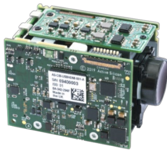
Figure 1. Harrier USB/HDMI Interface Board mounted on a MP1110M camera (J1 – KEL cable not connected)
