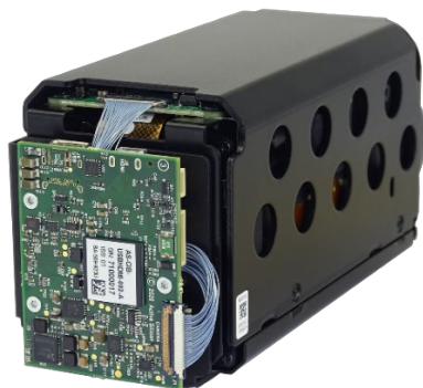
Figure 3. Harrier USB/HDMI Interface Board mounted on a MP2030-GS camera
