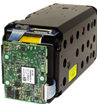
Figure 3. Harrier USB/HDMI Interface Board mounted on a Harrier 36x AF-Zoom Camera with global shutter
