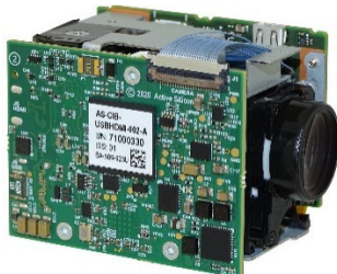
Figure 1. Harrier USB/HDMI Interface Board mounted on a Tamron MP3010M-EV camera
