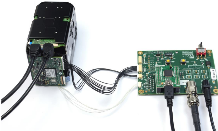
Figure 7. Harrier Evaluation Board connected to Harrier USB/HDMI Camera Interface Board and FCB-EV7520A camera.
