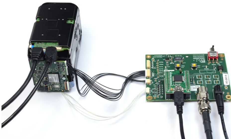
Figure 8. Harrier Evaluation Board connected to Harrier USB/HDMI Camera Interface Board and FCB-EV7520 camera.
