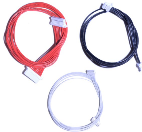
Figure 5. Harrier Evaluation Board cables
