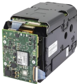
Figure 1. Harrier USB/HDMI Interface Board mounted on a FCB-EV7520A camera
