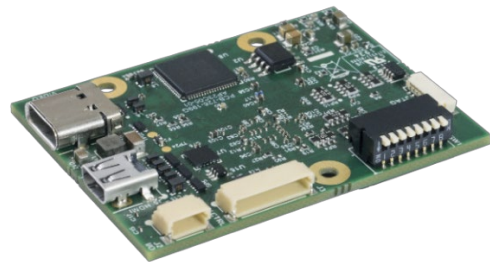
Figure 2. Reverse side of Harrier USB/HDMI Camera Interface Board
