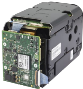
Figure 1. Harrier USB/HDMI interface board mounted on a Sony FCB-EV7520 with connecting 30-way micro coax KEL cable
