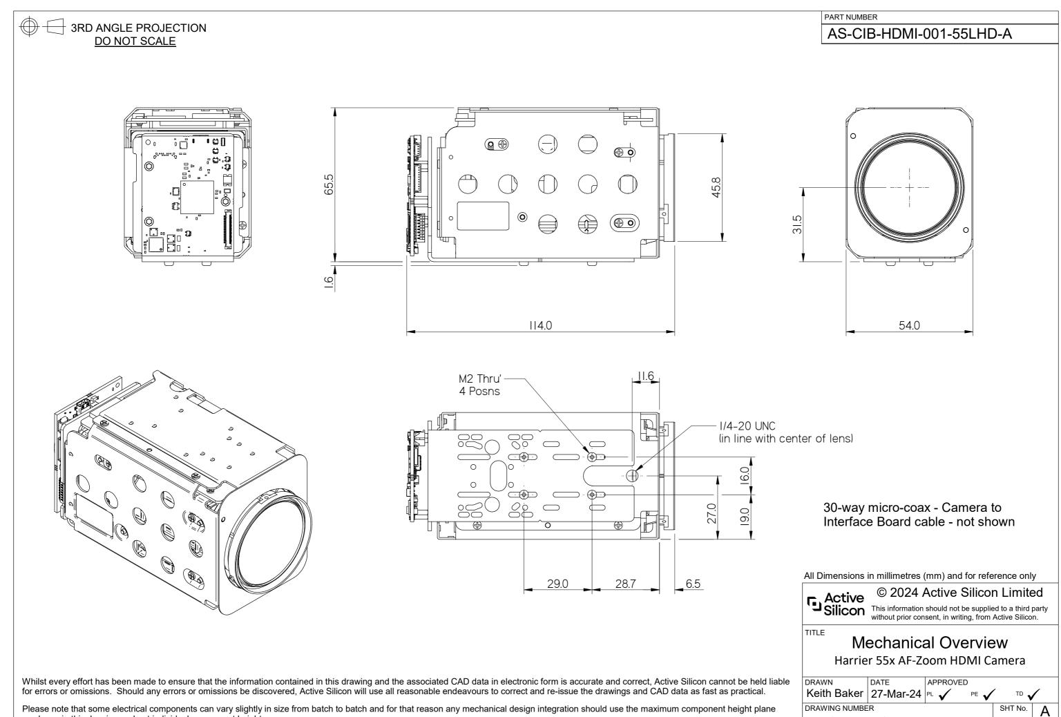
Please note that some electrical components can vary slightly in size from batch to batch and for that reason any mechanical design integration should use the maximum component height plane as shown in this drawing and not individual component heights.
