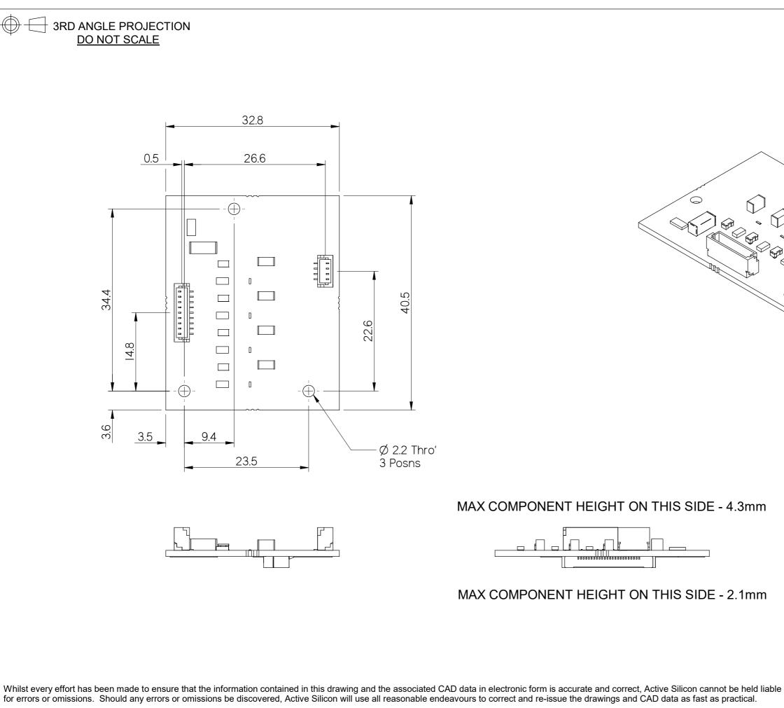
Please note that some electrical components can vary slightly in size from batch to batch and for that reason any mechanical design integration should use the maximum component height plane as shown in this drawing and not individual component heights.
