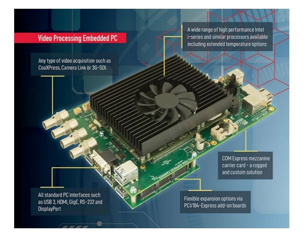
The pictured Video Processing Embedded PC, or one of our other embedded systems, can be easily adapted to a multitude of medical or industrial applications.
