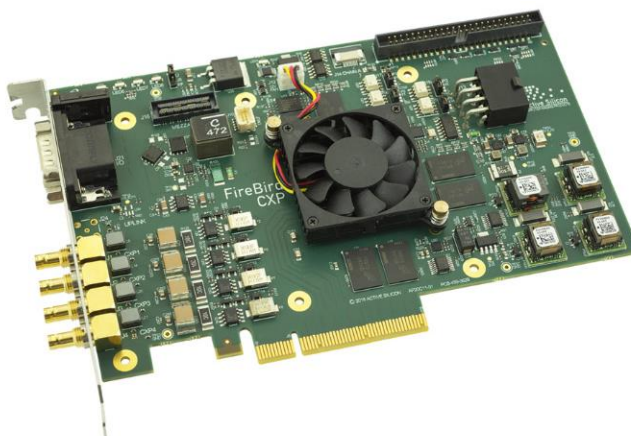
Active Silicon's new FireBird CoaXPress frame grabber 4xCXP-12 PCIe Gen3 x8
