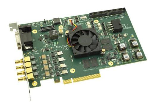
Active Silicon's FireBird CoaXPress frame grabber 4xCXP12-3PE8 supports v2.0
