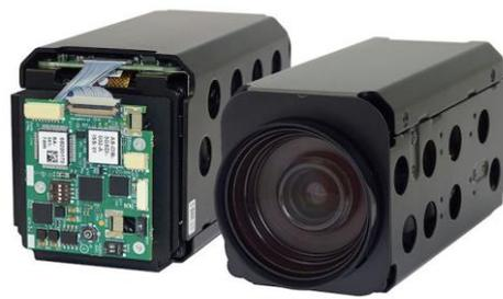
Our [HD-SDI AF-Zoom Block Camera](#) with Tamron MP2030M-GS combines the high-quality CMOS sensor of the Tamron with our advanced [Harrier processing technology](#), delivering HD-SDI (1080p/30, 720p/60) output as well as HD-VLC™ compressed video for very long cable length applications. This makes the camera ideal for mounting in inaccessible areas and is a perfect solution for motion-sensitive applications such as traffic monitoring, ANPR and toll station use.
