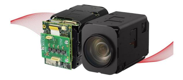
The camera is a direct replacement for the FCB-EV7520/A series with the same dimensions and offering several improvements, including higher low-light visibility and a Super Image Stabilizer. It features several advanced functions like Spot Focus, ICR, color image acquisition, Wide Dynamic Range and many more.
