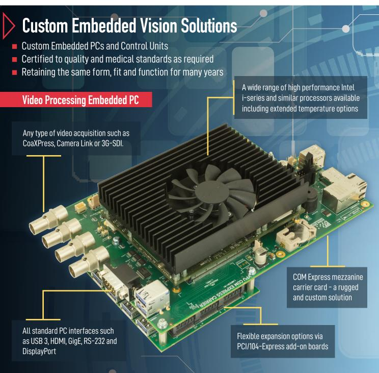
Active Silicon custom embedded systems are designed for specific OEM applications such as medical devices, industrial automation, process control, security and others.
