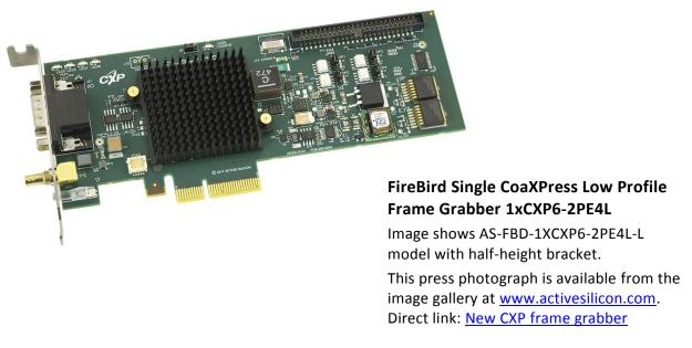
The low-profile design of this FireBird Single CoaXPress frame grabber allows the board to be used in small 2U enclosures; a full-height bracket is also available for standard PC cases. It is a
