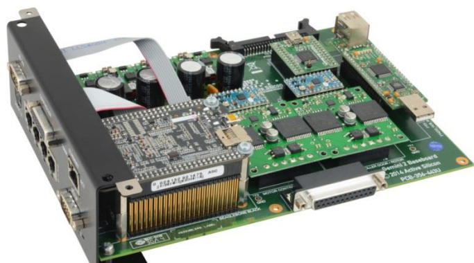
Figure 2 | ARM based embedded vision system for an industrial machine application
