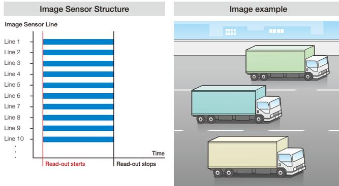
A "Global Shutter CMOS Image Sensor" allows capturing target images without any artifacts by running the scan on all the scan-lines simultaneously. "Global Shutter CMOS Sensor" that effectively eliminates the imaging artifact with excellent image rendition of fast moving objects.
