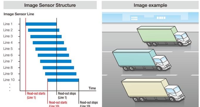
A "Rolling Shutter CMOS Sensor," as employed in general camera modules, captures target images sequentially from upper to lower scan-lines; artifacts are incurred on fast moving objects (focal plane distortion) due to the sequential delay to run each scan.
