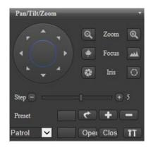
Figure 4. PTZ control panel
