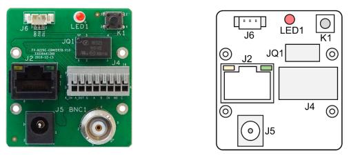
Figure 2. Harrier 23x/52x IP Camera Evaluation Board and Block Diagram
