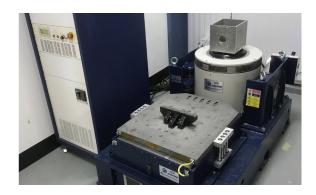
Incorporating a climatic chamber, vibration table, and altitude test chamber, we are able to test our products to exacting standards for shock, vibration, temperature and humidity. In addition, we can simulate the low pressure conditions of >50,000ft as required for some of our antenna units.
