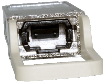
Figure 7. End-view of QSFP+ SR4 Optical Transceiver Showing "Male" Registration Pins
