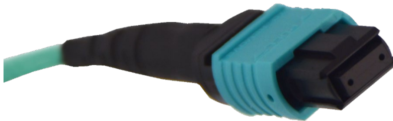
Figure 6. A Fiber Ribbon Cable with a Female MPO/MTP* Connector
